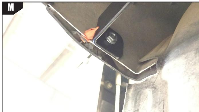
c. Reinstall the support bracket using the factory 10mm bolts and the supplied ¼" X ½" hex head bolt
