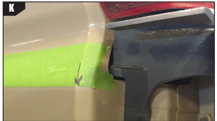
7. Stretch tape vertically under the tail light as shown (**Photo... Still need this photo**)
