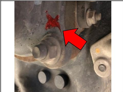
c. Carefully inspect the flat surface behind the axle nut to ensure the area is free of any weld spatter.
