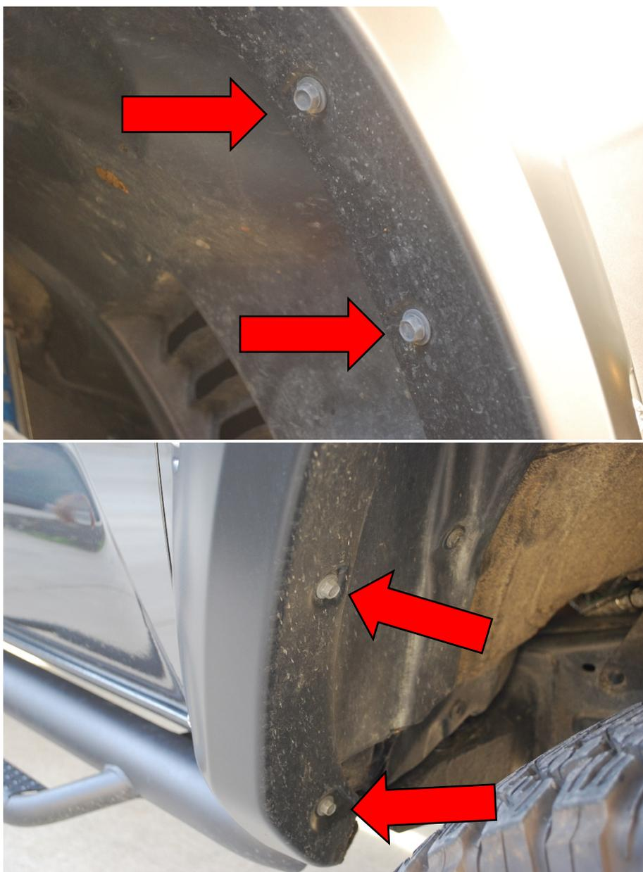
4. Remove 10mm bolts from the underside of the front bumper (this will vary depending on if you have the oem wind deflector still on etc.) otherwise you should have 4-6 bolts to remove.
