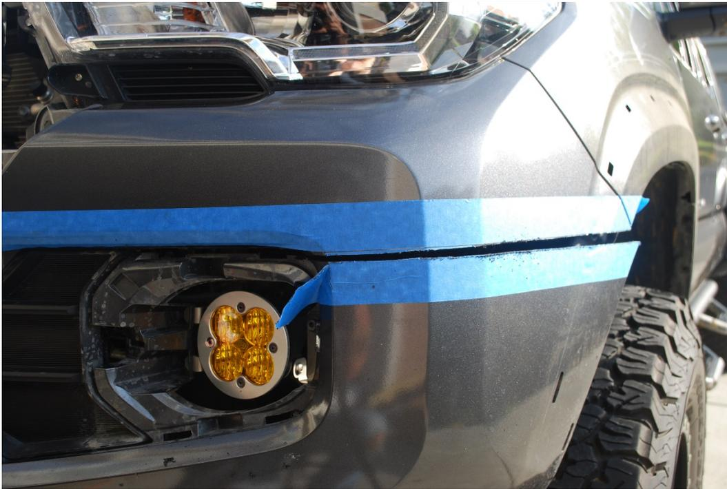
9. Once both sides have been cut, remove lower portion of bumper which has just been cut.
