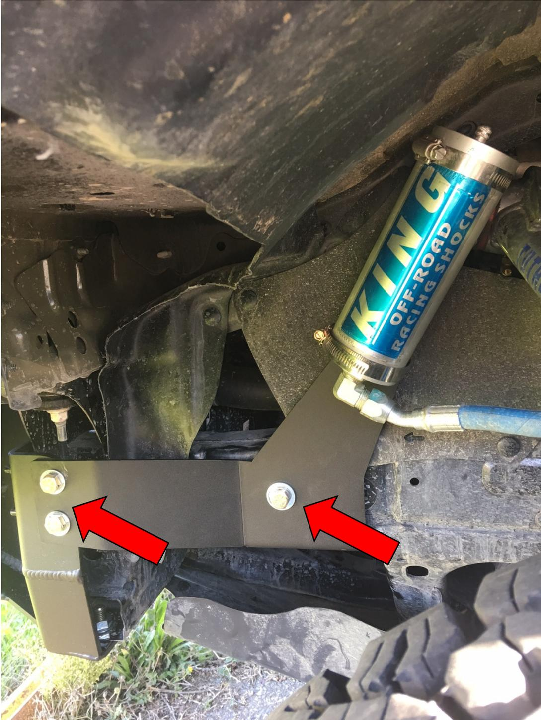
21. With everything hand tight, make final adjustments and place the last spacer, bolt, washer and nut combination on the bottom portion of the new front bumper on each side.
