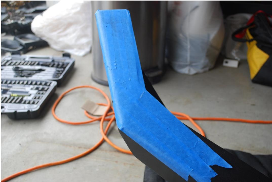
17. Place the bumper onto the 3 preexisting bolts from the oem crash bar. While in place use the oem nuts from earlier removal, along with the newly supplied washers and hand tighten them for now to allow minor fitment adjustments. You will ultimately want around  $\frac{1}{4}$ " + gap between the bumper and your cut bumper area to allow for any front bumper flex that may occur.
