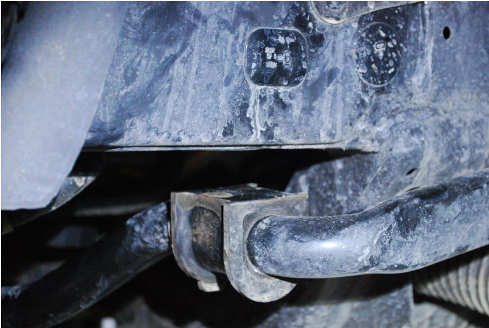
20. With the lower two bolts that were just removed from the sway bar mounts, re use along with newly supplied washers and mount the new side support bracket using the newly supplied hardware (7/16" x 4" long grade 8 bolt, round washer, nut and square zinc plated washer)
