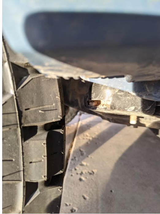
Figure 5: Clearances during the “stuff test”. a) Tire to fender flare. b) Tire to cab mount.
