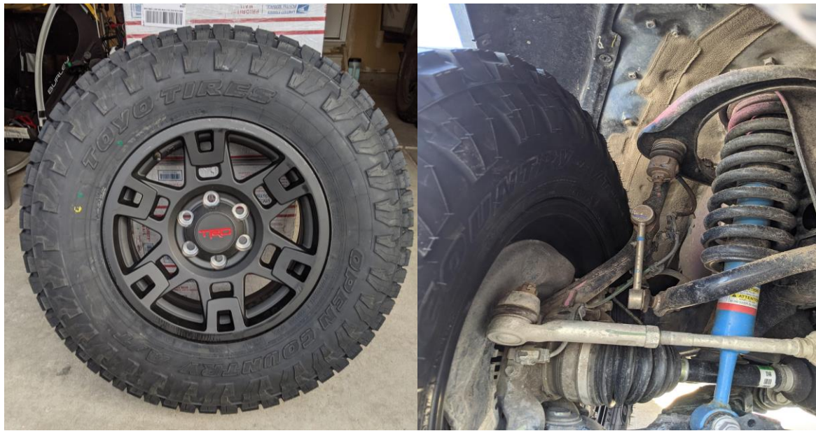
Figure 1 a/b: The tires/wheels and showing the space between the UCA.
