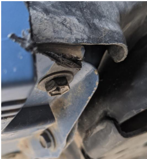
Figure 3: Bottom view of the rear part of the wheel well fender that was cut.
