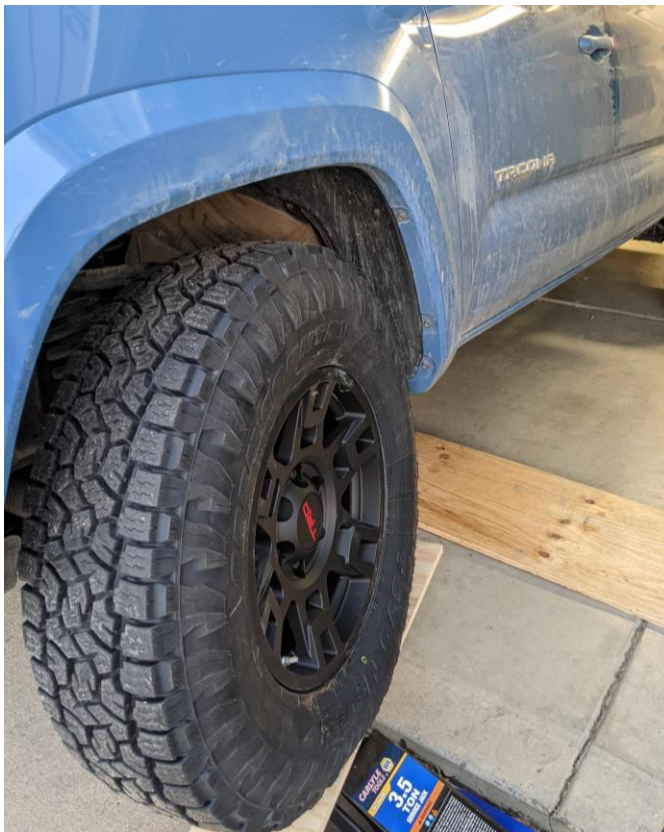
Figure 6: The position of the tire during the “stuff test” when it was closest to the fender flare.
