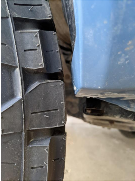
Figure 5: Clearances during the “stuff test”. a) Tire to fender flare. b) Tire to cab mount.
