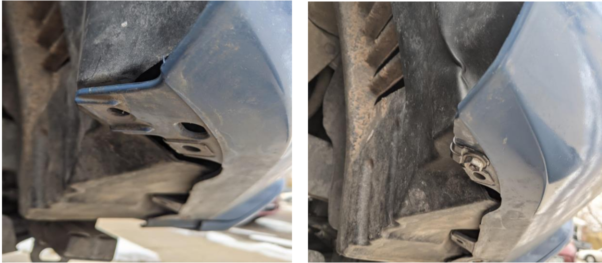
Figure 4: Front part of the wheel well a) before and b) after cutting.
